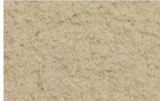
RF - INDICATIVE RENDER WALL FINISH Limewashed finish on lime render. Colour TBC.
